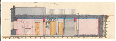
Existing Kew drawing section - note the first floor structure to be removed is a later addition
